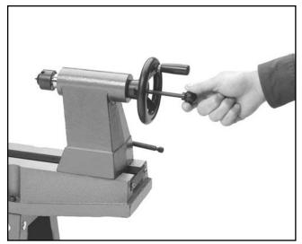
Figure 14. Removing live center.
